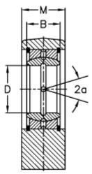
Α = 55 a (degrees) = 7 В = 20 D = 25 Dynamic load C (kN) = 48F = 45 L = 72.5 = 23
